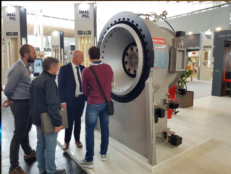
Wood powder burner 16 MW
