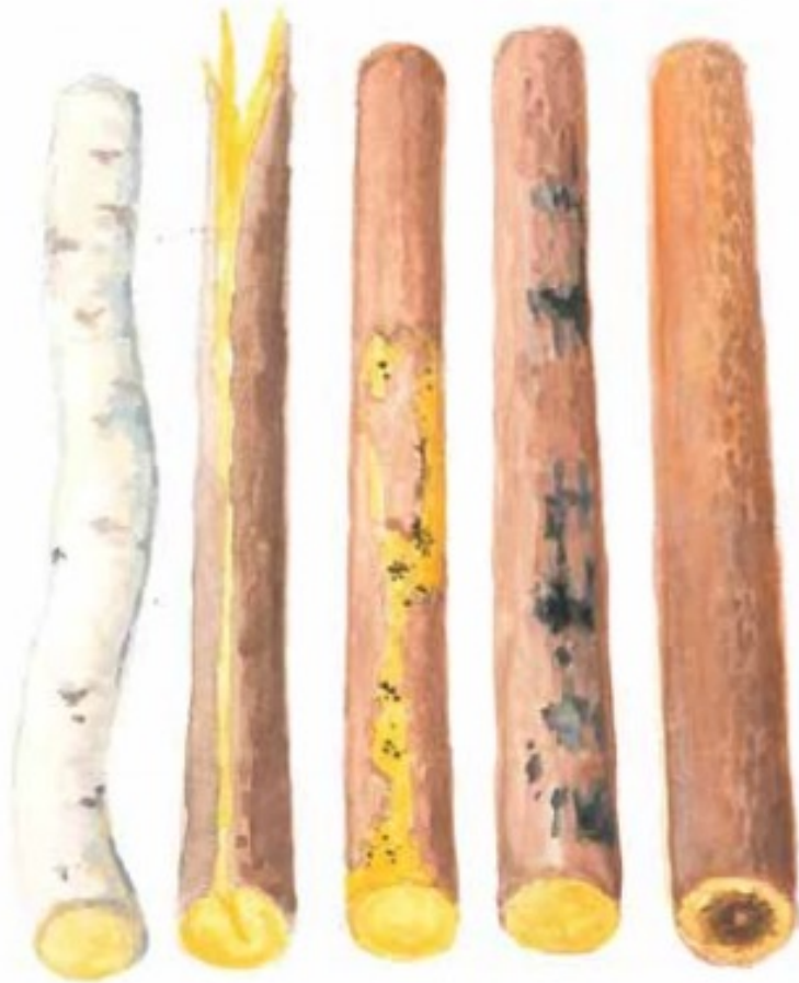
Examples of discarded wood. Crooked stem. Splinted stem. Insect infested stem. Fire damaged, charred stem. Rotten stem.
