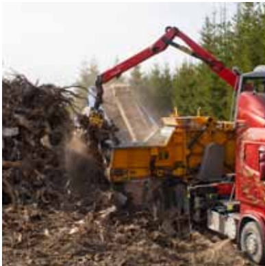
A large crusher from Allan Bruks AB handling stumps in the forest.
