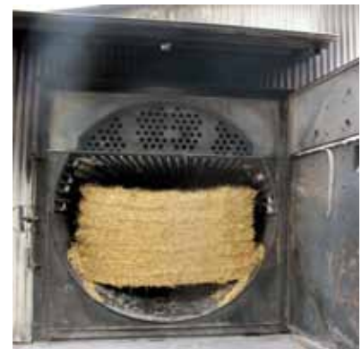
Straw bales and other farm residues are often burnt in cylindrical boilers.
